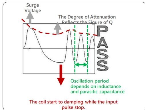
Detect Layer Short by Compare Damped Oscillation Waveforms
